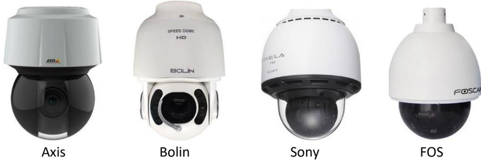
In each case the dome camera hangs from an arm and typically offers 360° capabilities. Higher end cameras will offer continuous rotation; some cheaper models will have a stop point. All dome cameras will have a limit that prevents them from pointing very far above the horizon (if at all) – some offer from 15° to 20° above the horizon. This is an important factor in your decision-making process, and we come back to this later.
